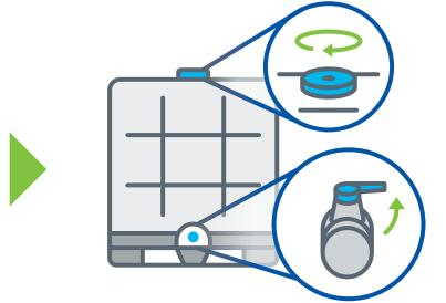
**CLOSE VALVE AND TIGHTEN FILL CAP**
