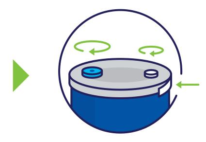
TIGHTLY CLOSE REMOVABLE LID, FILLING AND VENT HOLES (BUNGS), AND RE-SECURE THE RING WITH BOLT AND NUT
