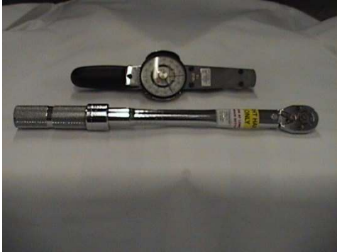
Dial Indicating and Adjustable Torque Wrench
