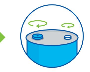
**TIGHTLY CLOSE ALL FILLING AND VENT HOLE OPENINGS (BUNGS)**
