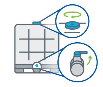
**DO NOT REMOVE OR MASK ORIGINAL CONTENT LABELS**  **EMPTY CONTENTS UNTIL DRIP DRY &/OR NO MORE THAN 1 INCH OF NON-POURABLE MATERIAL REMAINS NO MATERIAL SHOULD REMAIN AT THE BOTTOM OR IN THE CORNERS OF THE IBC**
